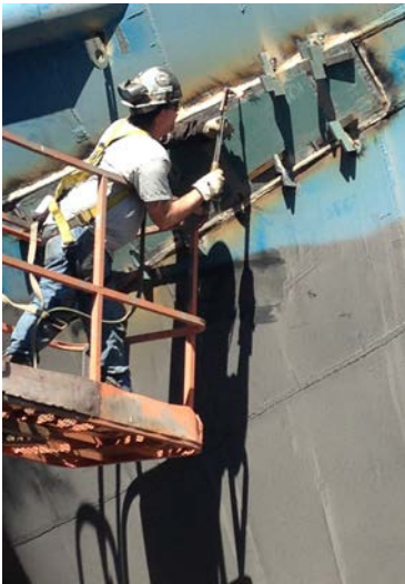
Fabricator, Sean Baker hard at work installing an insert on the hull of the FV Fleeton
